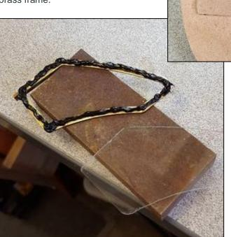
For this I have used a RTV silicone black which when cured will look very much like the rubber seal on the full size, RTV is used as it will stick with a strong bond to both the brass frame and alass window. it can also withstand very high heat. It can if needed. also be easily cut away with a sharp scalpel. BTW the slides are 3"x 2"x 1 mm thick
