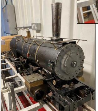
With the cab removed attention was then focused on what is best described as the tender but in reality, is a water tank and bunker on the rear end of the loco frames.
