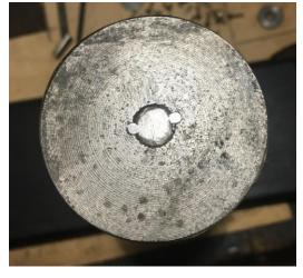
dismantled John gave all the components a really good clean. The die block in the expansion link was needed a new pin but apart from that all was now good.
